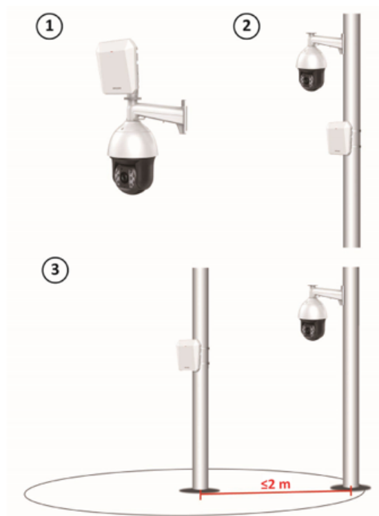
Figure 10-18 Scenario of One-Point Calibration
